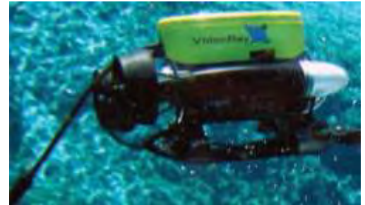
Figure 23: Remotely Operated Vehicle Used for Underwater Investigations
