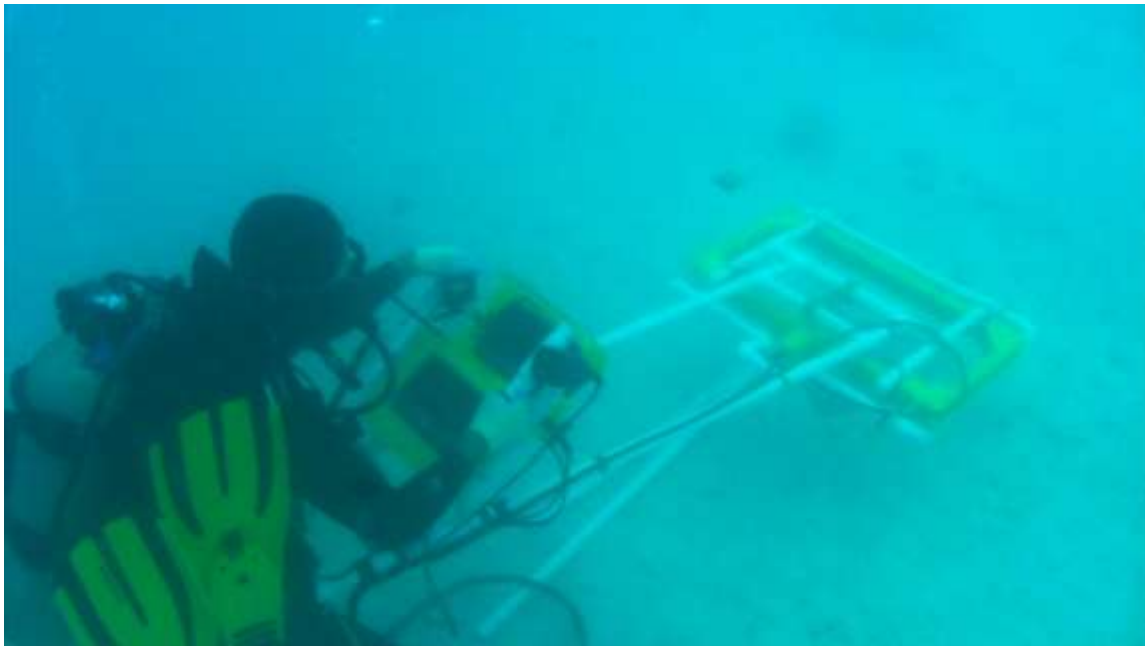
Figure 35: Diver Using an Electromagnetic Device on a Sled
