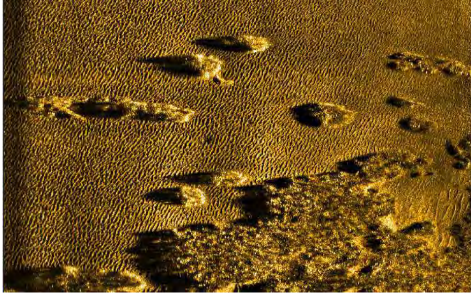
Figure 25: Example of Side Scan Sonar Showing Underwater Features
